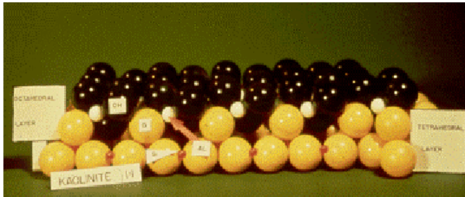
Figure 3.8 Kaolinite clays are composed of one layer of silica and one layer of alumina.
